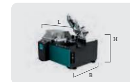
CUBO 300 NC BOX B 2030 mm L 1830 mm H 1830 mm h 870 mm Kg 900
