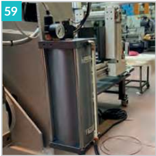
000947 Minimal lubrication system 3 liters
